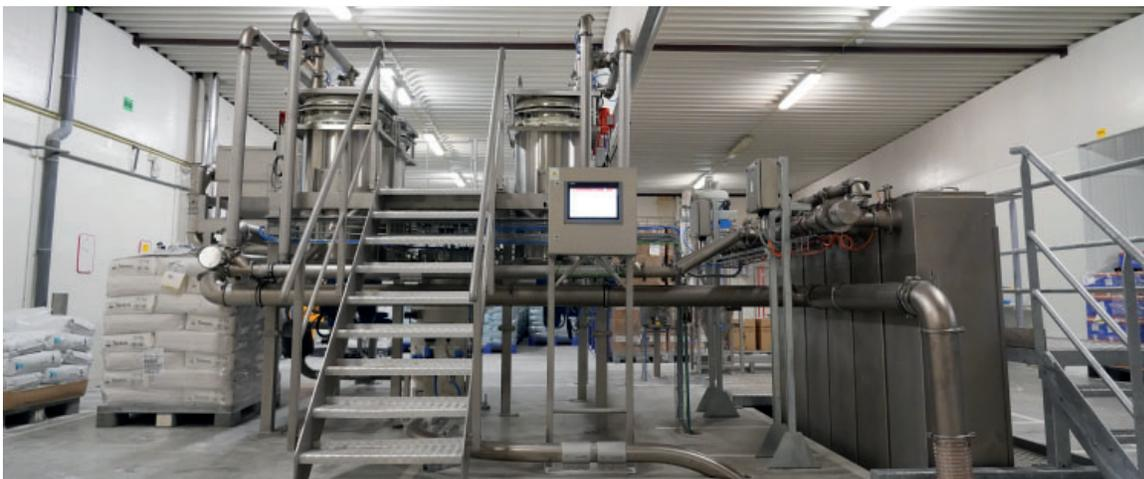
*Climate-controlled tanks, transportation pipes, weighing and dosing equipment, and mixers are controlled by a fully configurable recipe management and production control system.*
