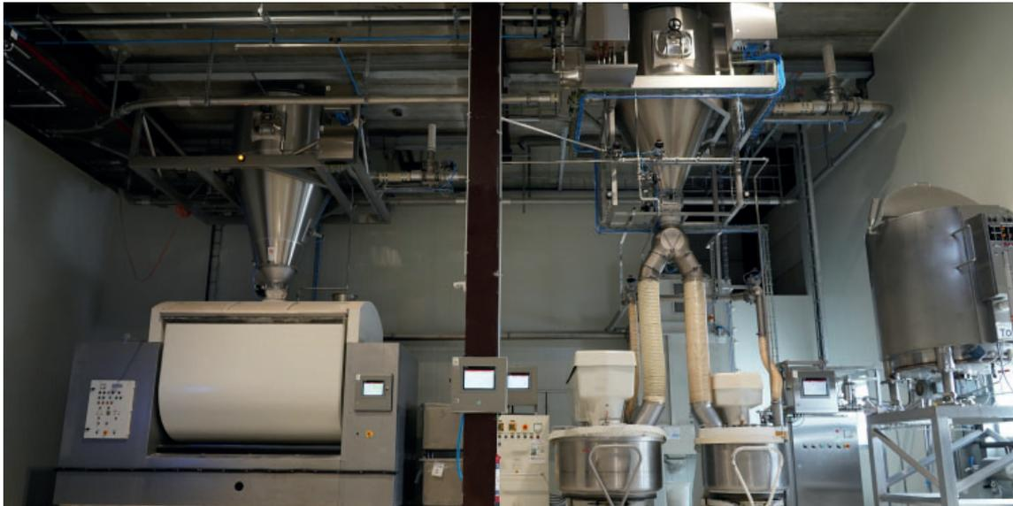
*The dough chambers are equipped with a convenient dust extraction system, making for a much more pleasant work environment.*
